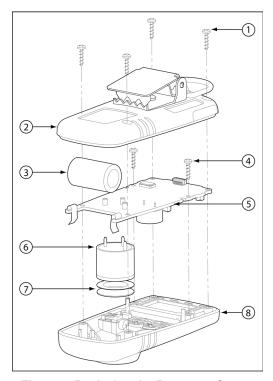
Figure 4. Replacing the Battery or Sensor
