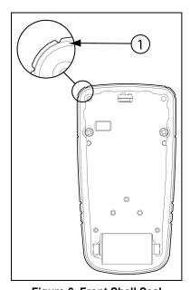
Figure 6. Front Shell Seal Table 13. Front Shell Seal
