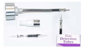
• In order to use the new VOC zeroing tubes and adapter, the instrument <u>must</u> be equipped with a **Flex-I-Probe** inlet.
