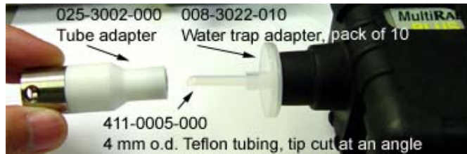
Connection to Multi-gas monitors
