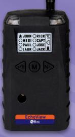
The EchoView Host is a mini-controller that creates a self-contained intelligent wireless network that supports up to 8 monitors. The easy-to-read display allows connected devices' names to be customized for easy identification of the real-time readings. The EchoView Host provides immediate remote notification of alarm conditions to keep workers informed, connected and protected.
