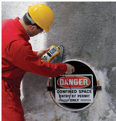
Confined space testing with the MultiRAE Lite
