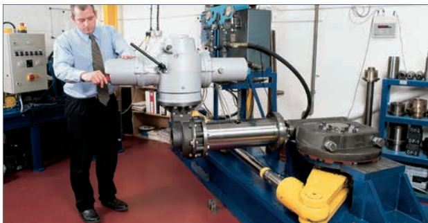
Endurance testing of prototype subsea gearbox.
