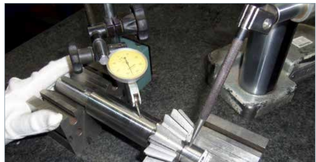
Concentricity test with dial indicator.
