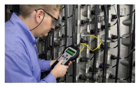
The hand-held UV Intensity sensor monitor allows operators to quickly and easily measure duty and reference sensor calibration.
