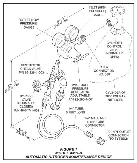
**Step B.** Inspect the Cylinder Control Valve outlet for dirt, dust, damaged threads, oil, or grease. Remove dirt and dust with a clean cloth. If damaged threads, oil, or grease are present, replace the cylinder.
