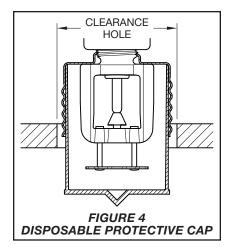
Step 5. Replace the Protective Cap by pushing it upwards until it bottoms out against the Support Cup. See Figure 4. The Protective Cap helps prevent damage to the Deflector and Arms during ceiling installation and/or finish. You can also use the Protective Cap to locate the center of the clearance hole by gently pushing the ceiling material up against the center point of the Protective Cap.
