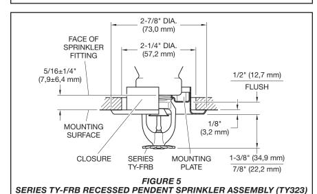
WITH TWO PIECE 1/2 INCH TOTAL ADJUSTMENT STYLE 20 RECESSED ESCUTCHEON
