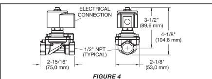
212 PSI (15,0 BAR) MAXIMUM SERVICE PRESSURE SOLENOID VALVE IN-SERVICE NORMALLY CLOSED & ENERGIZED
