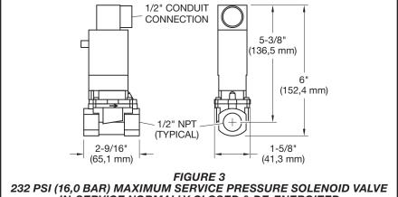
IN-SERVICE NORMALLY CLOSED & DE-ENERGIZED (ENERGY PULSE TO OPEN SUBSEQUENT ENERGY PULSE TO CLOSE)
