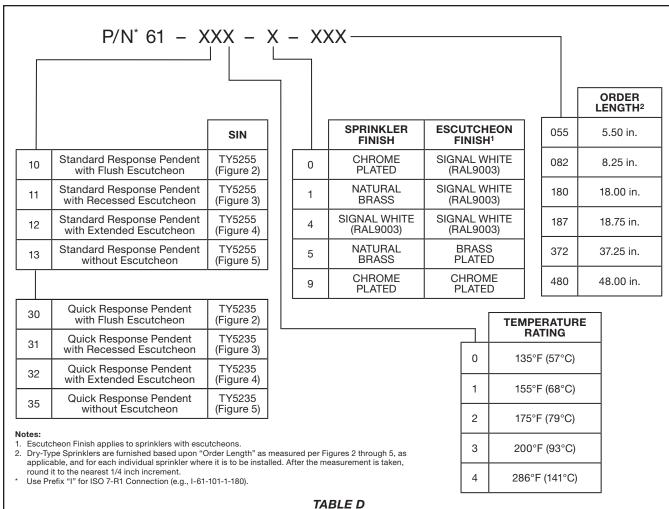
TABLE D SERIES DS-2 STANDARD AND QUICK RESPONSE, STANDARD COVERAGE, DRY-TYPE SPRINKLERS PART NUMBER SELECTION
