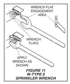
Close the fire protection system control valve and drain the system before removing the sprinkler.
