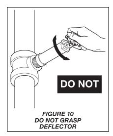
**Note:** If sprinkler removal becomes necessary, remove the sprinkler using the same wrenching method noted above. Sprinkler removal is easier when a non-hardening sealant was used and torque guidelines were followed. After removal, inspect the sprinkler for damage.
