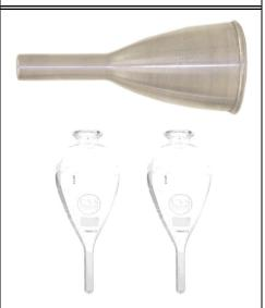
CVS Centrifuge Tube: **Model # 45243- 100**, 100mL **Short Cone** Made to API Standards, and graduated as follows:
