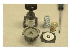
3. Remove and inspect the Diaphragm Assembly (11) from the Lower Body Assembly (1).
