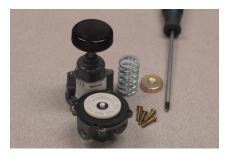
2. Remove Qty. 4, screws (17) holding the Spring Case (2) and the Body Assembly (1) together. Lift off the spring case, and remove the Spring (5), and Upper Spring Seat (6)
