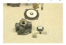
4. The Inlet Filter (13), Plug (12), and Spring (14), can be accessed by first removing the Filter Plug (16) using a 1" wrench or similar
