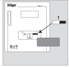
Remove the cover of the Polytron 3500, by gently pulling apart the cover on both sides and lifting upwards.
