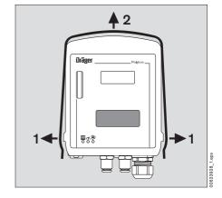
Fit the Polytron 3500 using the metal hooks into the slots provided on the docking station.
