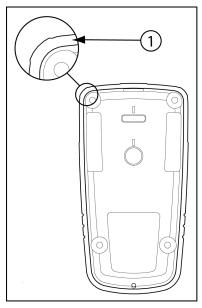
Figure 5. Rear Shell Seal
