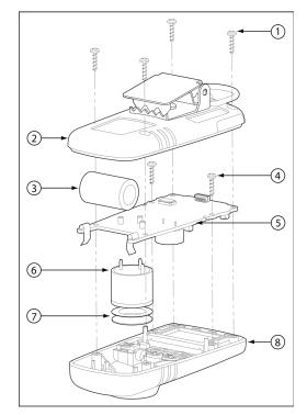
Figure 4. Replacing the Battery or Sensor
