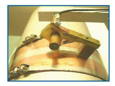
The effectiveness of JOWA - PES must continuously be controlled to keep the propeller protected. The voltage meter monitors permanent the present condition with output signal to alarm system.
