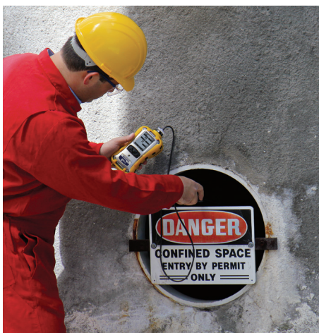
Confined space testing with the MultiRAE Lite
