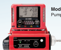
SDM-2009 Stand alone calibration station
