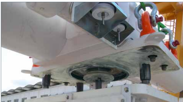
Actuator declutch system.
