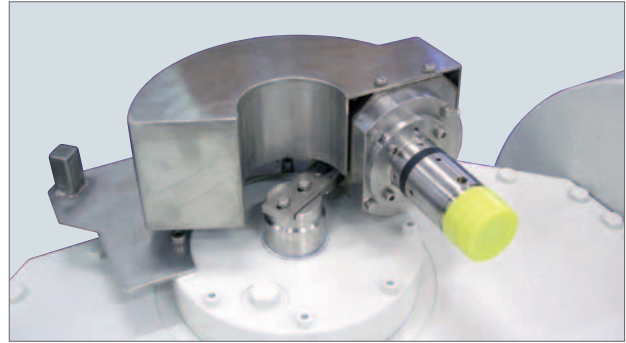
Position transducer assembly with electrical instrumentation connector.
