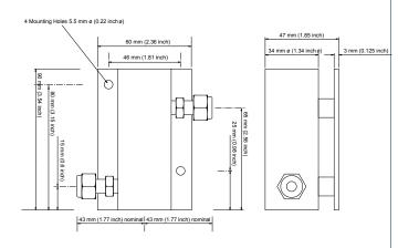
NOTE: The assembly is shown with ½ inch OD tube fittings. The dimension across the tube fittings will vary for all other size fittings.
