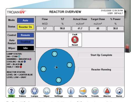
The TrojanUVSwift controller is equipped with a robust PLC and touchscreen display configured for user-friendly operation. The system provides dose pacing for optimized disinfection performance and communicates with plant SCADA systems for centralized monitoring.
