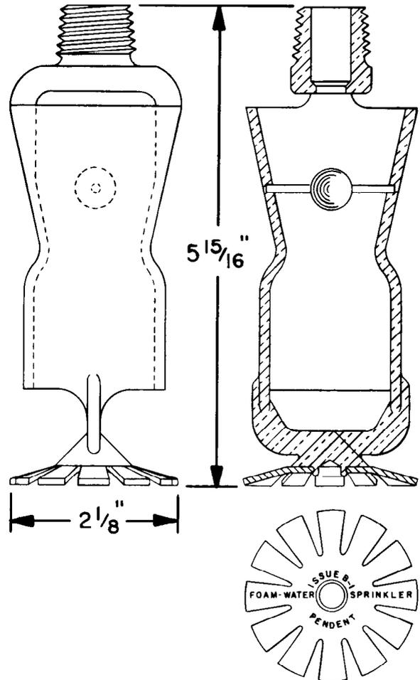
CONNECTION: 1/2" NPT OR FINISHED FOR 1/2" (.840" O.D.) BRAZED CONNECTION. FURNISHED WITH 1/2" NPT UNLESS OTHERWISE SPECIFIED.
